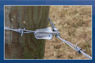
The Gripple T-Clip Barb is engineered for use on  $12^{1/2}$  gauge (2.50mm) mild steel barb wire and 14 gauge (2.00mm) high tensile barb. For thinner,  $15^{1/2}$  gauge (1.70mm) high tensile barb wire, use the standard Gripple T-Clip, that can also be used to terminate stock fence.
