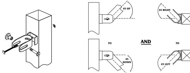
Stainless steel is 75,000 PSI yield strength. Bracket will not fracture on severe impact as will cast material. Bracket allows simultaneous 45° rotation side to side and up and down.
