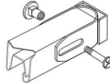
One-way fastener cannot be loosened by normally available tools.
