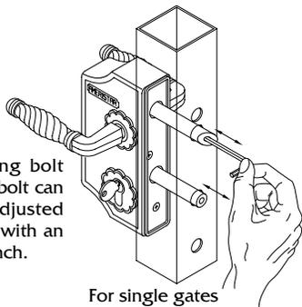
Self-latching bolt and dead bolt can both be adjusted over 3/8" with an Allen wrench.
